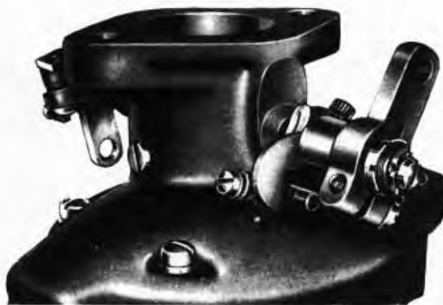
Fig. S-21 Spring-Loaded Governor Lever
